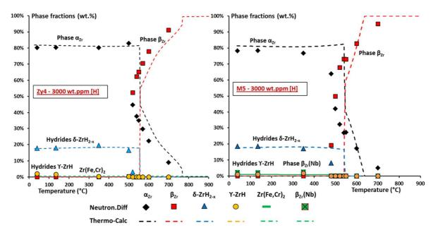
Figure 1: Evolution of phase weight fractions as a function of temperature obtained by neutron diffraction (symbol) *in situ* during step-cooling from 700°C and thermodynamic calculations (dotted curves) for Zircaloy-4 (left) and M5 (right) containing about 3000 wt.ppm of hydrogen
