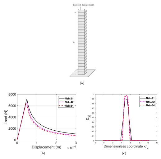
Figure 5: The finite element mesh for the three-dimensional bar (a). The uniaxial responses (b) and the damage profiles (c) for different meshes: Nel=21,42 and 84.
