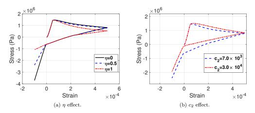
Figure 3: Effect of the parameter  $\eta$  and the constant  $c_2$  on the uniaxial response.
