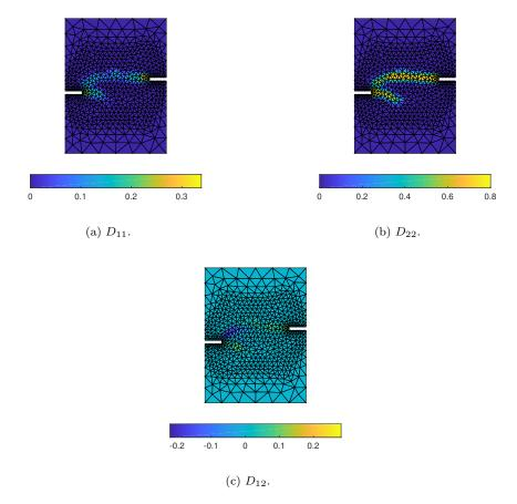
Figure 12: Damage is ovalues for each component in the neighborhood of the notches for  $\eta=0.$
