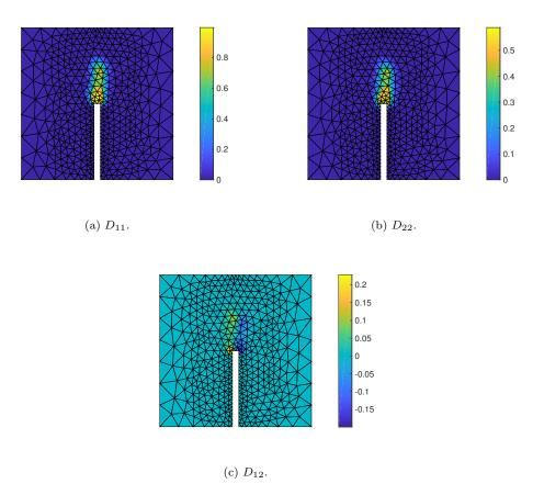
Figure 10: Damage is ovalues for each component for  $\eta=0.$
