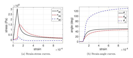
Figure 8: Stress and angle evolutions for Willam's test using the proposed model.
