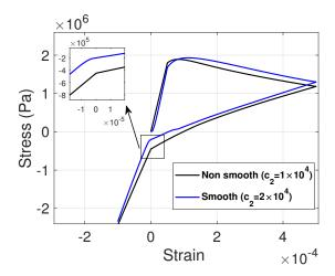
Figure 2: Effect of the regularity of the opening (closure) cracking functions on the uniaxial response.
