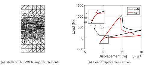
Figure 11: Finite element mesh and reaction curve (Shi's test).
