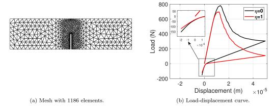
Figure 9: Finite element mesh and reaction curve (three point bending test).
