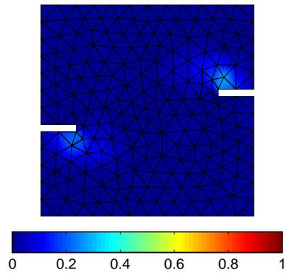
Figure 10: Damage isovalues for each component in the neighborhood of the notches (Shi test).
