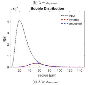
Figure 4: Impact of the regularization parameter on the estimation of the bubble size distribution N(a). Dotted black curve: input distribution. Red dashed curve: result of Tikhonov regularization. Blue dashed curve: smoothed curve
