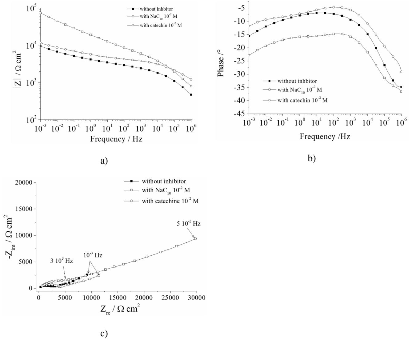
Figure 7: Impedance diagram of “metal/CL” system in ASTM corrosive water without and with corrosion inhibitors after 24 hours of immersion. (a, b) Bode representation, (c) Nyquist representation.
