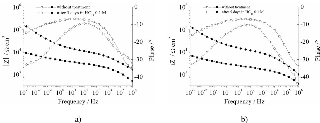
Figure 13: Impedance diagram of “metal/CL” system without and with  $\text{HC}_{10}$ -based conversion treatment (5 days in  $\text{HC}_{10}$  0.1 M) after (a) 48 h and (b) 480 h of immersion in ASTM corrosive water.
