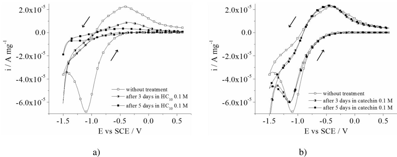
Figure 9 : Voltammogram of lepidocrocite in CPE in  $\text{Na}_2\text{SO}_4$  0.1 M electrolyte without treatment and after immersion in (a)  $\text{HC}_{10}$  solution and (b) catechin solution
