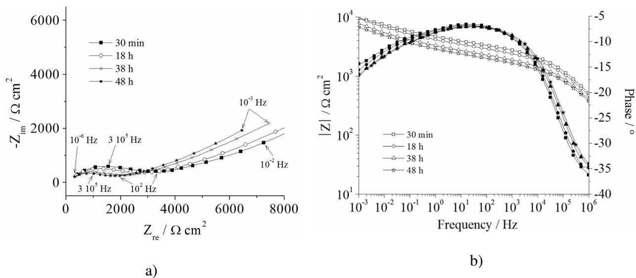
Figure 5: Impedance diagram of “metal/CL” system in ASTM corrosive water at different immersion time in (a) Nyquist representation and (b) Bode representation.
