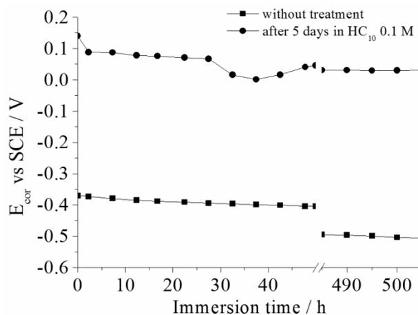
Figure 12: Corrosion potential measurements of “metal/CL” system versus immersion time in ASTM corrosive water without treatment and after  $\text{HC}_{10}$ -based conversion treatment.
