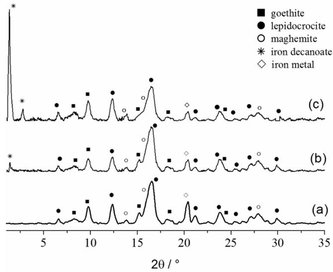
Figure 2: X-ray diffractograms of corrosion layer without inhibition treatments (a), after 5 days of immersion in  $\text{NaCl } 10^{-2} \text{ M}$  solution (b), after 5 days of immersion in  $0.1 \text{ M HCl}$  solution (c)
