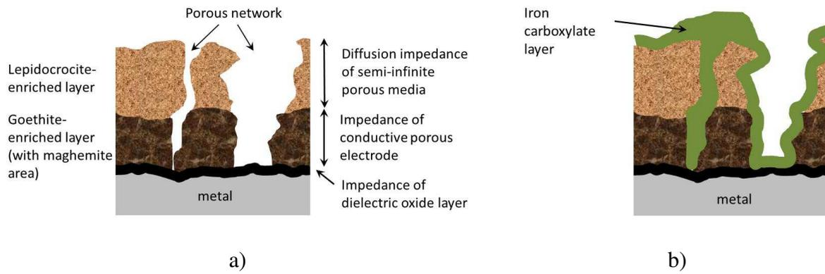
Figure 6: (a) Schematic structural model of the “metal/CL” system, (b) HC<sub>10</sub>-treated structure of “metal/CL” system
