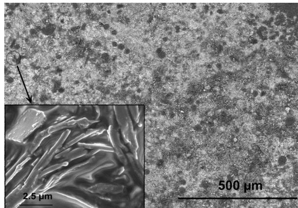
Figure 11: SEM observation of surface of CL after HC<sub>10</sub>-based conversion treatment (5 days in HC<sub>10</sub> 0.1 M) in BSE mode and zoom of iron carboxylate deposit in SE mode
