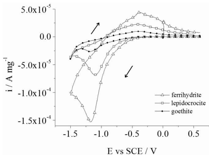
Figure 8: Voltammogram of different iron oxyhydroxide phase in CPE in  $\text{Na}_2\text{SO}_4$  0.1 M electrolyte
