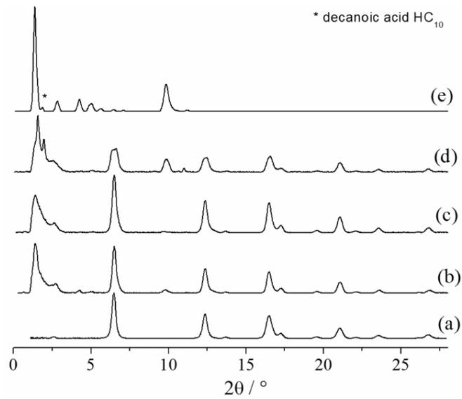
Figure 10 : X-ray diffractogram of lepidocrocite without treatment (a), lepidocrocite treated with HC<sub>10</sub> solution for (b) 1 day, (c) 3 days, (d) 5 days, and (e) synthesized iron decanoate from [36].
