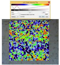
Fig. 2. Map of the Raman  $T_{2g}$  intensity line (fake colors) obtained on  $U_{0.75}La_{0.25}O_{2-x}(100x100 \mu m)$
