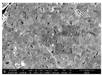
Fig. 1. SEM picture of the  $U_{0.75}La_{0.25}O_{2-x}$  sintered pellet
