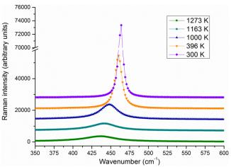
Fig. 2. Variation in the Raman spectra (T<sub>2g</sub> line) of CeO<sub>2</sub> with temperature in air
