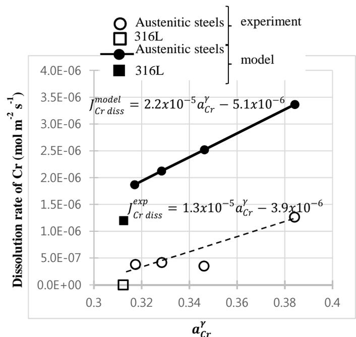
**Fig 4:** experimental and modelled corrosion rate of austenitic alloys in liquid Pb-Bi.
