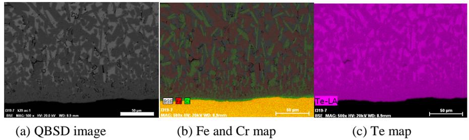
**Fig 5:** SEM-QBSD image of cross section of 316L after immersion in the melt for 30 min.
