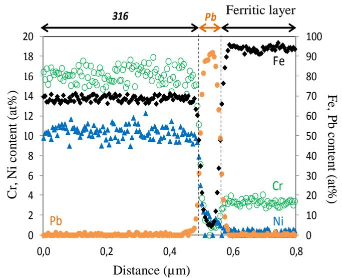
**Fig 3:** TEM-EDX profile of 316L sample corroded 1470 h in Pb-Bi at 500°C.
