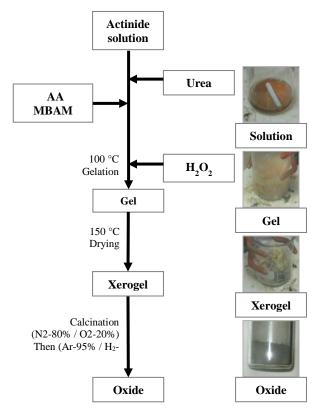
Fig. 1. Flowsheet of "advanced thermal denitration in the presence of organic dditives" synthesis route (photos illustrate the case of the  $(U,Pu)O_{2\pm\delta}$  synthesis).
