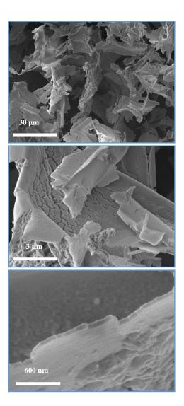
Fig. 4. Scanning electron images  $U_{0.55}Pu_{0.45}O_{2\pm\delta}$  converted for 2h at 800 °C in reconstituted air and then under hydrogenated argon (Ar-95% / H<sub>2</sub>-5%) for 2h at 800 °C
