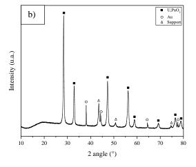
Fig. 3. XRD diagram for a)  $U_3O_8$  / PuO<sub>2</sub> converted for 2h at 800°C in reconstituted air and b) (U,Pu)O<sub>2</sub> converted for 2h in Ar-95%/H<sub>2</sub>-5%. Peak matches with white squares match the plutonium oxide phase, black stars match the uranium phase, black squares uranium-plutonium phase, white circles match the golden phase and white triangles match the support phase.
