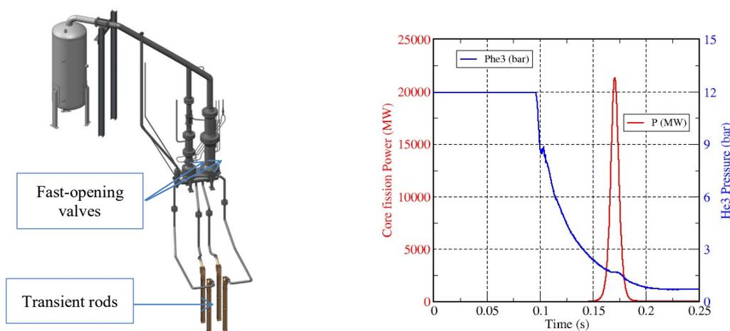
Figure 7 - Global view of the transient rods system (left) and of the typical CABRI <sup>3</sup>He Pressure and core power shapes during a RIA transient (right).
