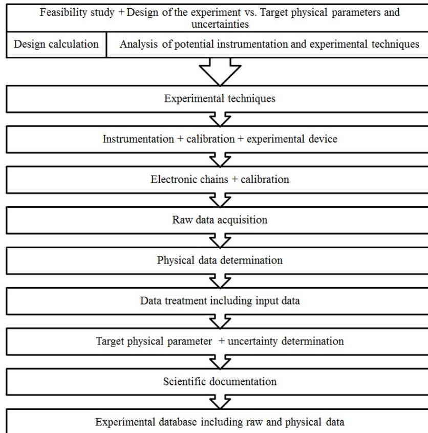
Figure 3 – Overall process to complete an experiment
