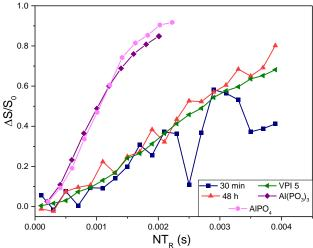
Figure 7. <sup>27</sup>Al {<sup>31</sup>P} REDOR curves of the 30 min- and 48 h-old samples compared to those of reference compounds.
