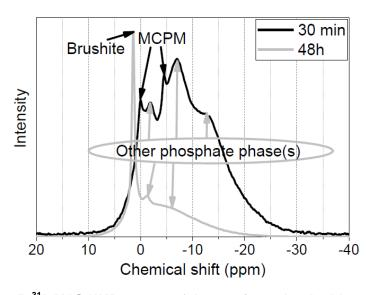
Figure 5. <sup>31</sup>P MAS-NMR spectra of the 30 min- and 48 h-old samples.
