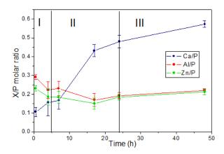
Figure 4: Evolution of the Ca/P, Al/P and Zn/P molar ratios (determined by SEM-EDS analysis) of the amorphous phosphate phase.
