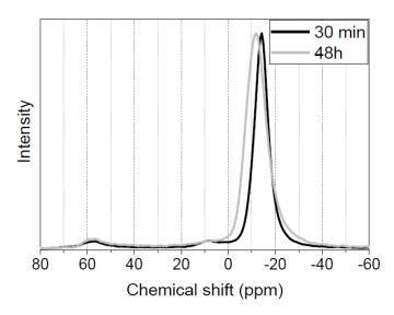
Figure 6. <sup>27</sup>Al MAS-NMR spectra of the 30 min- and 48 h-old samples.
