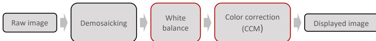
Figure 1. Color restitution flow from raw image to displayed image
