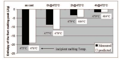
Figure 3: Simulated and measured incipient melting temperatures and enthalpies of the first melting peak during calorimetric heat up at a rate of 20  $^{\circ}C/min$ .
