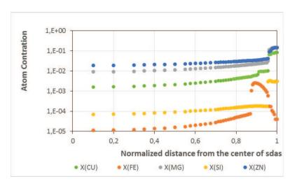
Figure 2: Simulated concentration gradients after solidification of aerospace alloy AA7449
