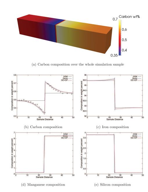
Figure 4: Simulated composition profiles after 10 days of tempering at 1050 °C, with experimental measurements by Darken [36] as circles.
