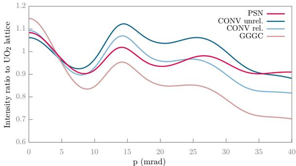
FIG. 1. (Color online) Ratio curves of the calculated momentum distributions of annihilating electron-positron pairs in  $V_U$  using different schemes. All spectra are convoluted with a Gaussian function with FWHM=4.7 mrad and divided by the lattice spectrum.
