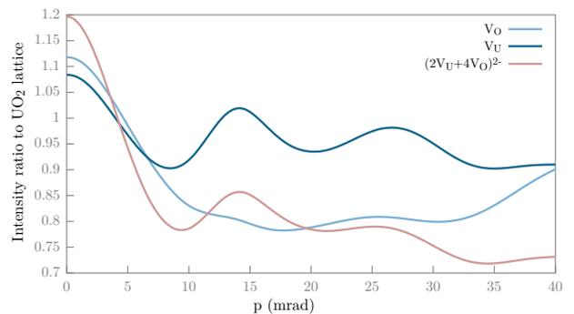
FIG. 3. (Color online) Ratio curves of the calculated momentum distributions of annihilating electron-positron pairs in various defects in  $UO_2$ . All spectra are convoluted with a Gaussian function with FWHM=4.7 mrad and divided by the lattice spectrum.
