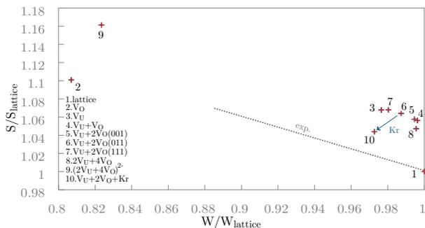
FIG. 7. (Color online)  $S_{\text{rel}}$  parameter as a function of the  $W_{\text{rel}}$  parameter plotted for various defects in  $\text{UO}_2$ , using windows  $S \in (0, 2.8)$  mrad and  $W \in (10.61, 26.35)$  mrad. The results were obtained using spectra convoluted with a Gaussian function with  $\text{FWHM}=4.7$  mrad. The arrow indicates the effect of krypton incorporation. The dotted line indicates the trend in the experimental measurements presented in Ref. 6.
