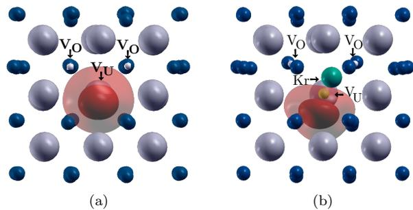
FIG. 6. (Color online) Positron isodensities (70% of the maximum density – solid and 30% – transparent), in red, found in the  $V_U+2V_O(110)$  defect, empty (a) and containing a Kr atom (b). Uranium atoms are presented in gray, oxygen atoms in blue and krypton in green. White and yellow spheres represent oxygen and uranium vacancies, respectively. Figures were generated using the XCRYSDEN<sup>41,42</sup> program.
