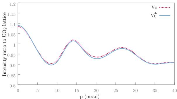
FIG. 4. (Color online) Ratio curves of the calculated momentum distributions of annihilating electron-positron pairs in  $V_U$  and  $V_U^{4-}$ . All spectra are convoluted with a Gaussian function with FWHM=4.7 mrad and divided by the lattice spectrum.
