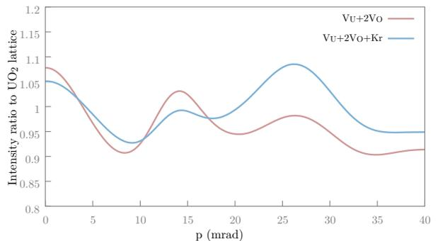
FIG. 5. Ratio curves of the calculated momentum distributions of annihilating electron-positron pairs in the  $V_U+2V_O(110)$  trivacancy (Bound Schottky Defect), empty and containing one Kr atom. All spectra are convoluted with a Gaussian function with FWHM=4.7 mrad and divided by the lattice spectrum.
