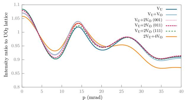
FIG. 2. (Color online) Ratio curves of the calculated momentum distributions of annihilating electron-positron pairs in various defects in  $UO_2$ . All spectra are convoluted with a Gaussian function with FWHM=4.7 mrad and divided by the lattice spectrum.
