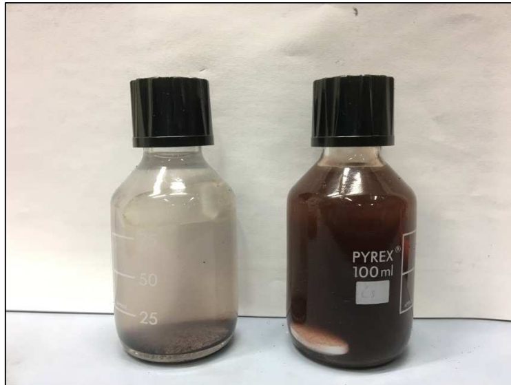
Figure 6 : Photograph of as-prepared Cu-HCF nanoparticles. Particles were prepared, dried, weighed, and then redispersed in water. Each bottle contains 1 g of Cu-HCF in 100 ml of commercially available mineral water, (composition in SI). The image was taken immediately after both samples were removed from the same rotary agitator. They had previously spent 4 days undergoing rotary mixing. . This far longer mixing time was used to remove any ambiguity. The bottle on the right had a magnetic stirring bar placed in it before rotary mixing began (batch 2). These particles were fully dispersed after 3 hours. The one on the left (batch 1) acted as a control contained a non-magnetic plastic object of similar size and shape to the stirring bar.
