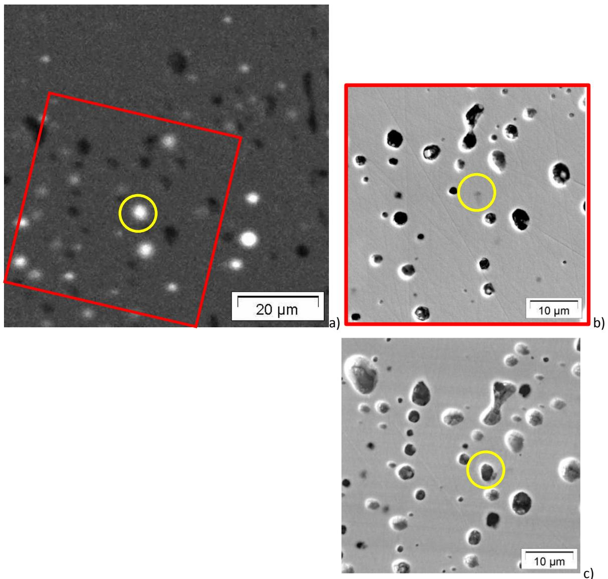
Figure 2: EMPA a) and Secondary electron images of the sample before b) and after c) sputtering. The bubble position lies inside the yellow circle. The red square in a) correspond to the image frame in b).
