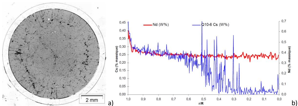
Figure1 : a)optical view of the analysed cross section b) Nd and Cs radial concentration profiles ( $r/R = 1$  at periphery,  $r/R=0$  at pellet centre)
