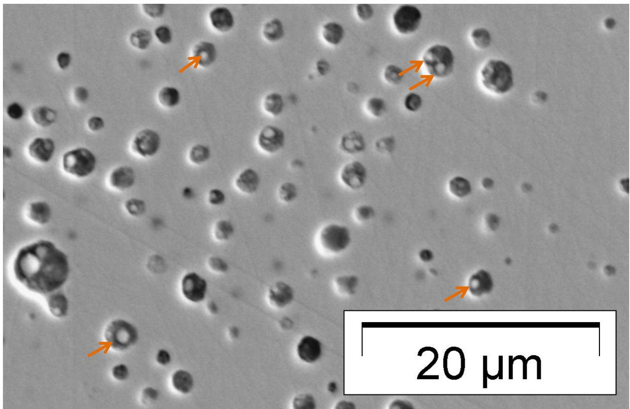
Figure 4 secondary electron image of the bubbles and the precipitates they contain (indicated by an arrow for some of them).
