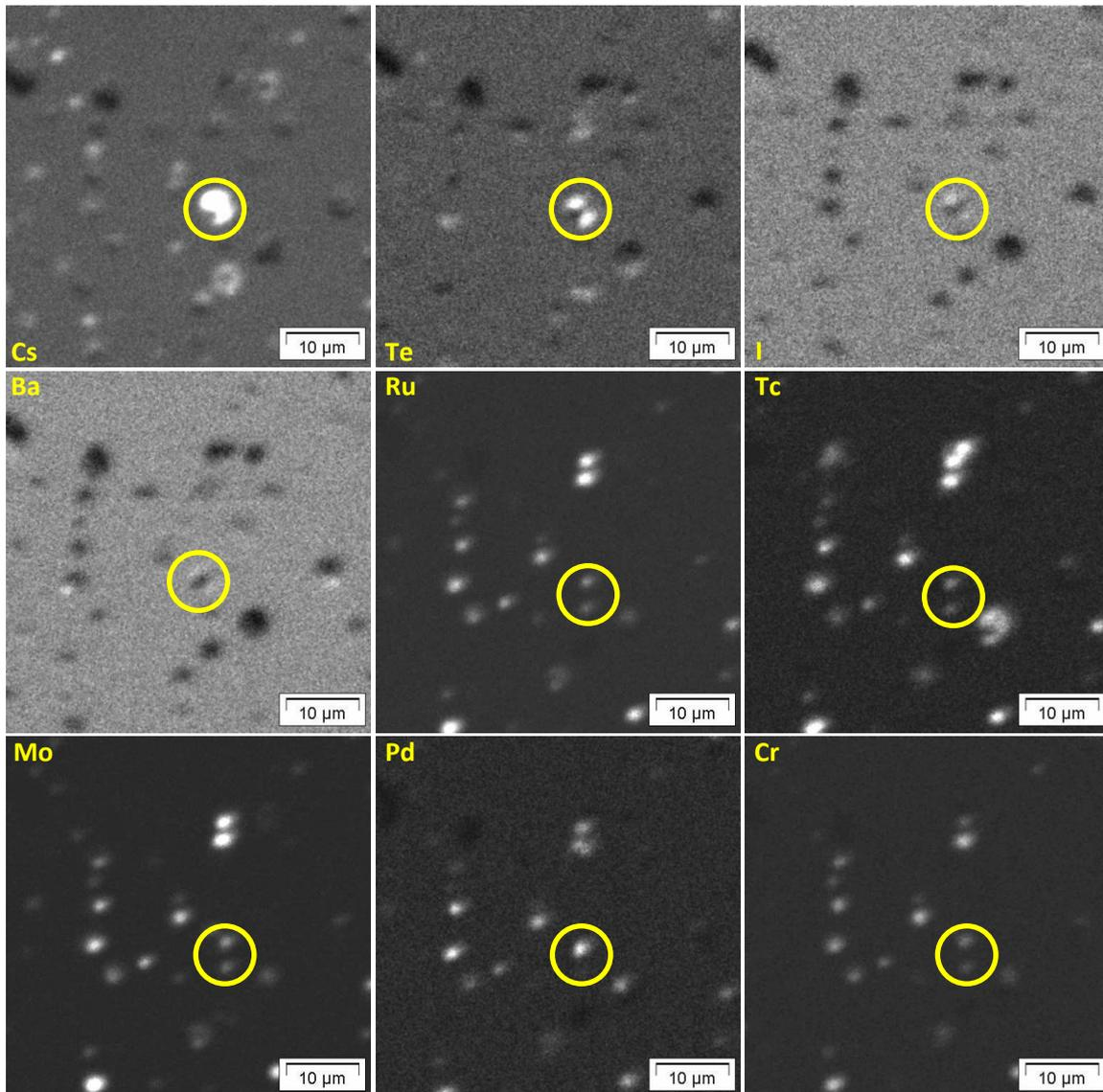
Figure 3: EMPA mapping of several fission products. The yellow circle corresponds to the bubbles identified in Figure 2.
