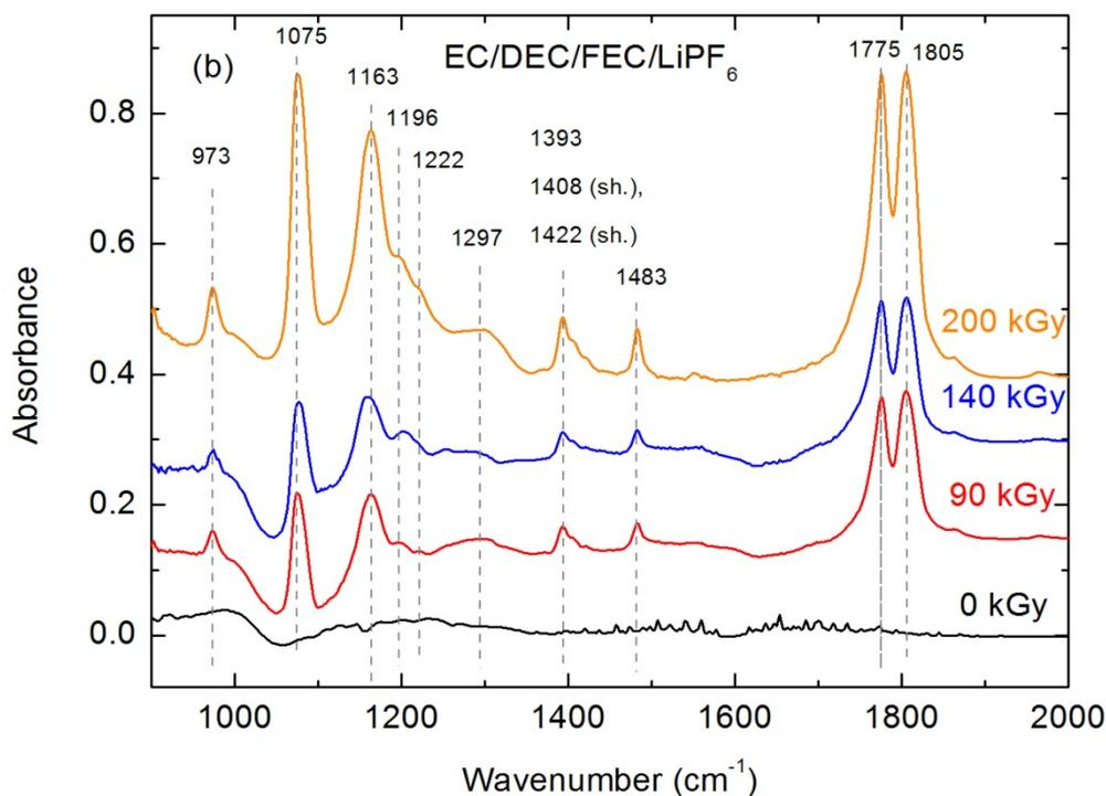
**Figure 3.** Evolution of IR spectra in the 900-2000  $\text{cm}^{-1}$  wavenumber range before and after irradiation at increasing doses for the Si NPs/electrolyte system: (a) EC/DEC/LiPF<sub>6</sub>; (b) EC/DEC/FEC/LiPF<sub>6</sub>. “sh.” stands for shoulder. The characteristic wavenumbers are displayed on the figures. As stated in the experimental section, no quantitative information can be obtained from these spectra. The spectra were thus rescaled for the sake of clarity.
