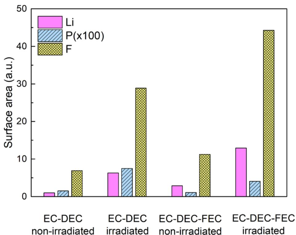
**Figure 2.** Evolution of the surface area corresponding to the elemental peak (PIXE P 2.013 keV; PIGE F: 197 keV and Li: 478 keV) for the Si NPs/electrolyte systems (with and without FEC) before and after irradiation at 200 kGy.
