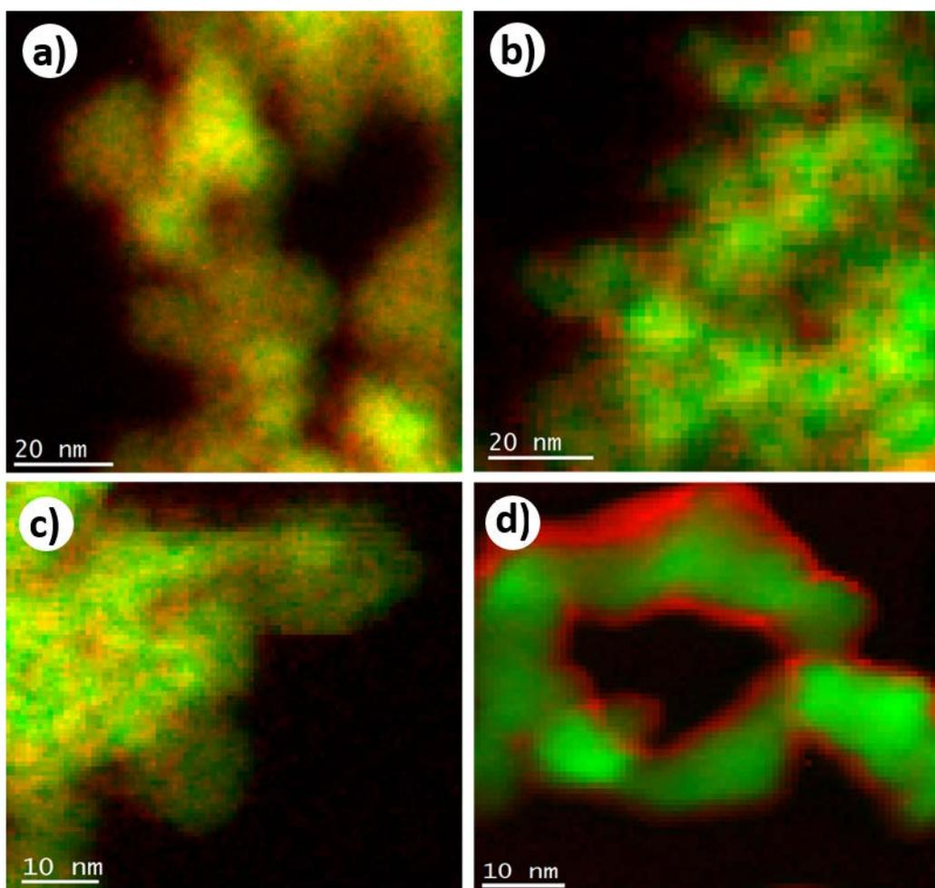
**Figure 6.** STEM images and EELS mapping of Si nanoparticles after (a) exposure to EC/DEC/LiPF<sub>6</sub> electrolyte; (b) irradiation at 190 kGy in a EC/DEC/LiPF<sub>6</sub> electrolyte; (c) exposure to EC/DEC/FEC/LiPF<sub>6</sub> electrolyte; (d) irradiation at 200 kGy in a EC/DEC/FEC/LiPF<sub>6</sub> electrolyte. The green color stands for silicon and the red one for carbon. The yellow color arises from regions with less carbon amount than the red ones.
