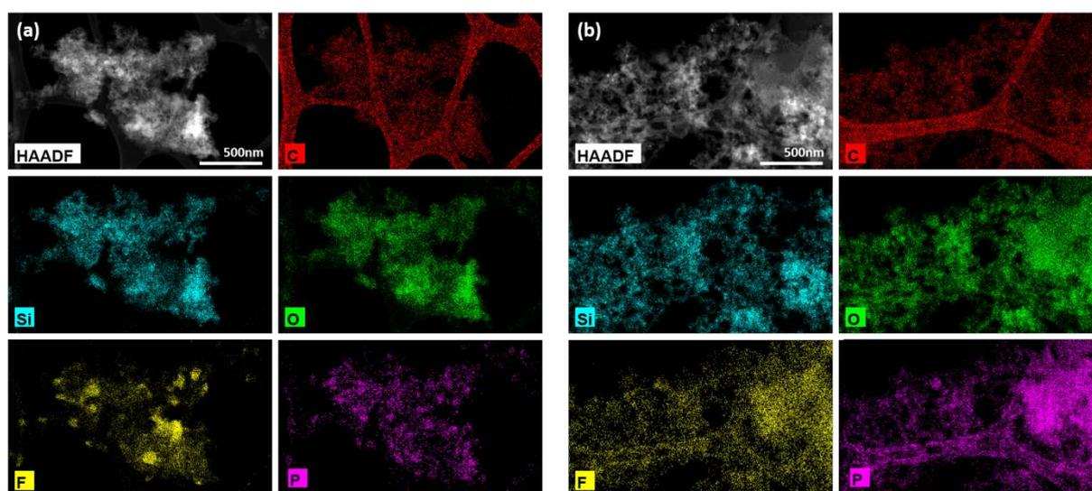
**Figure 4.** EDX images of the silicon nanoparticles (a) non-irradiated but exposed to EC/DEC/LiPF<sub>6</sub>; (b) irradiated at 200 kGy in EC/DEC/LiPF<sub>6</sub>. Carbon is in red; silicon in pale blue; oxygen in green; fluorine in yellow and phosphorus in purple.
