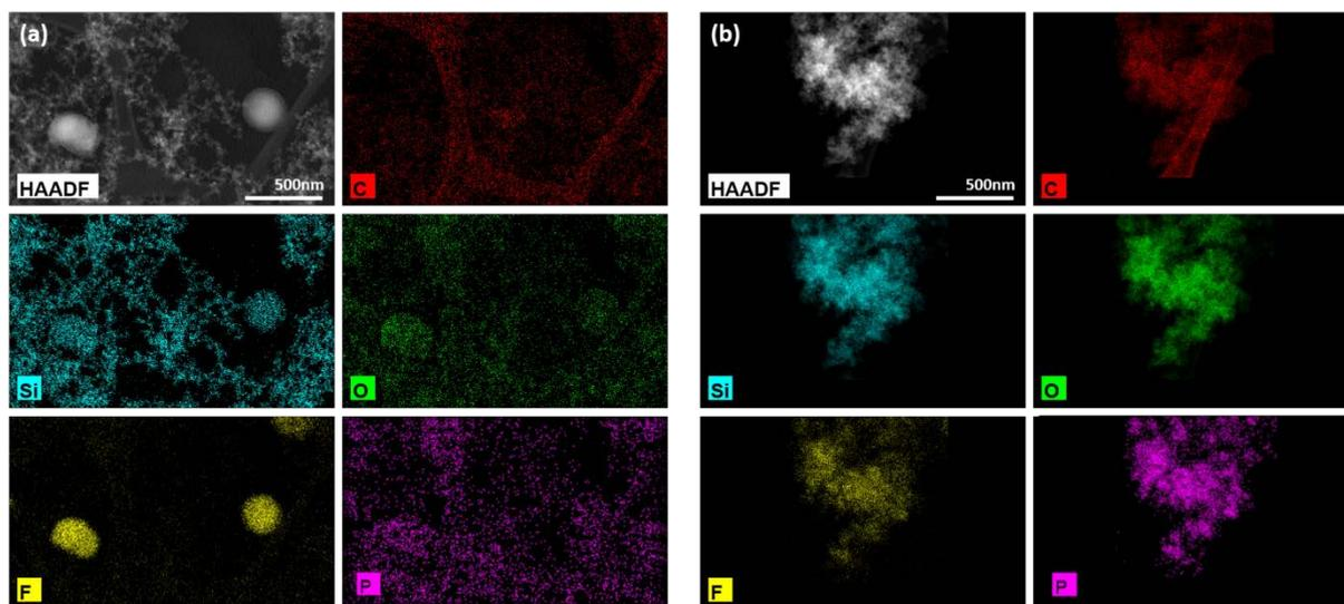
**Figure 5.** EDX images of the silicon nanoparticles (a) non-irradiated but exposed to EC/DEC/FEC/LiPF<sub>6</sub>; (b) irradiated at 200 kGy in EC/DEC/FEC/LiPF<sub>6</sub>. Carbon is in red; silicon in pale blue; oxygen in green; fluorine in yellow and phosphorus in purple.
