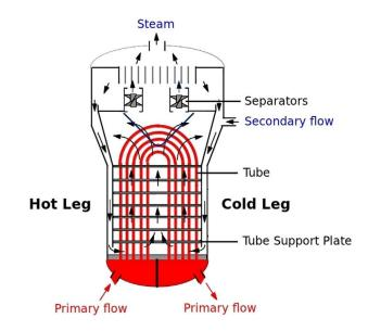
Figure 1: PWR recirculating steam generator [1]
