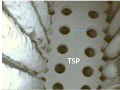
Figure 3: Photo of SG tube fouling [1].
