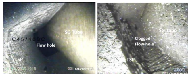
Figure 2: Photo of TSP clogging: top view of a « clean » flow hole on the left and an entirely clogged flow hole on the right side [1].
