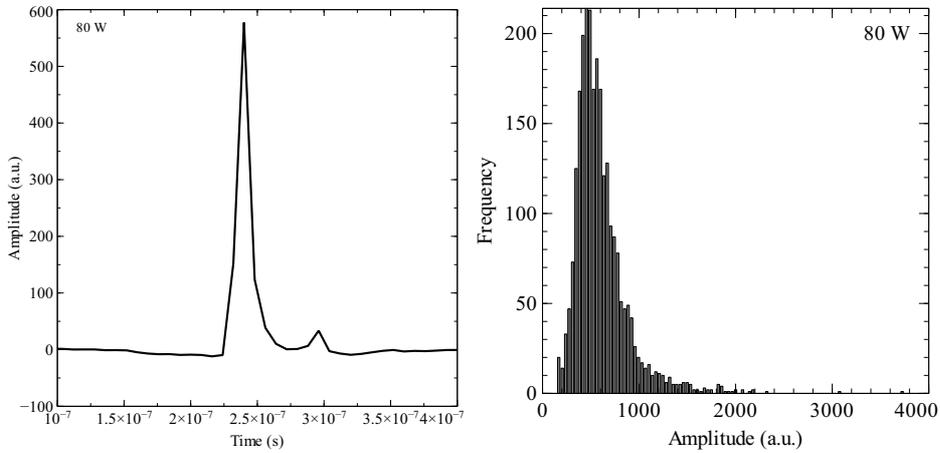
Figure 10: Left: mean pulse shape computed with single pulses coming from the 80 W measurement data. Right: amplitude distribution of pulses computed on datasets recorded at 80 W.
