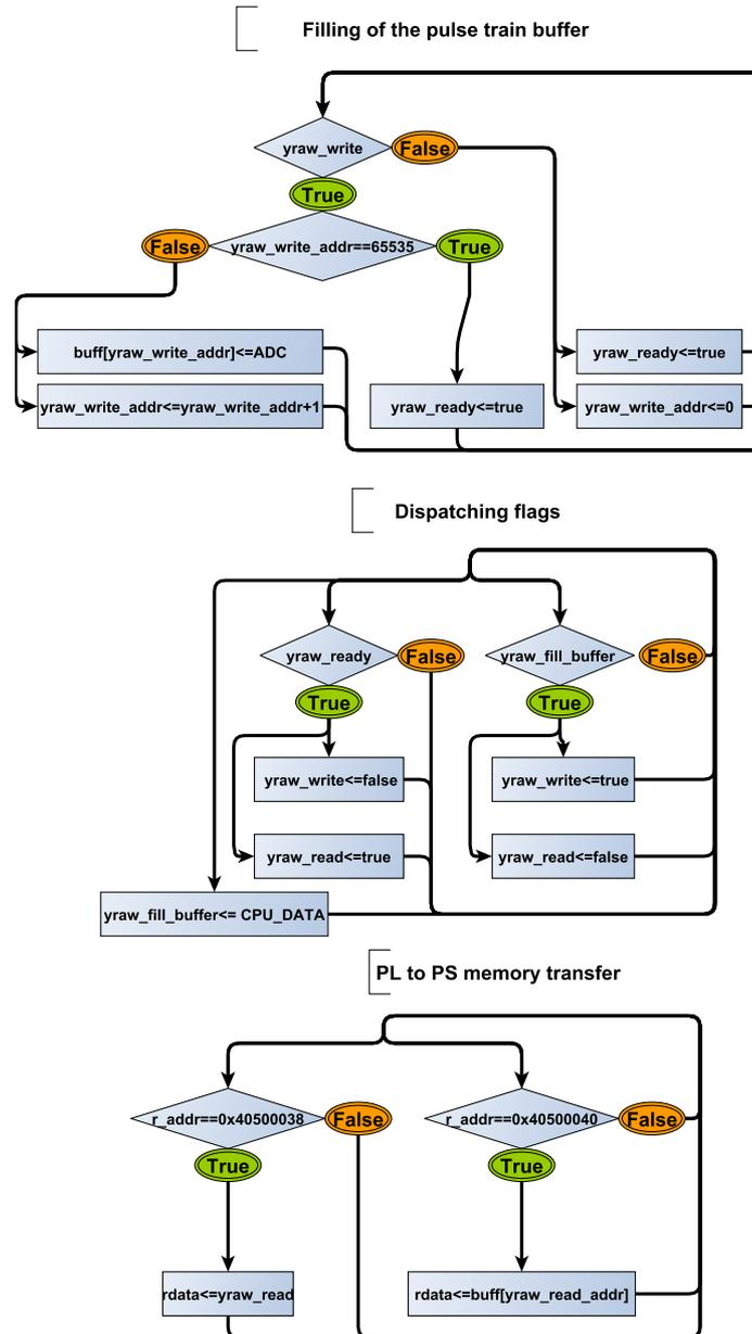
Figure 6: Smart detector algorithm implemented on the FPGA. The register ADC represents a raw sample.
