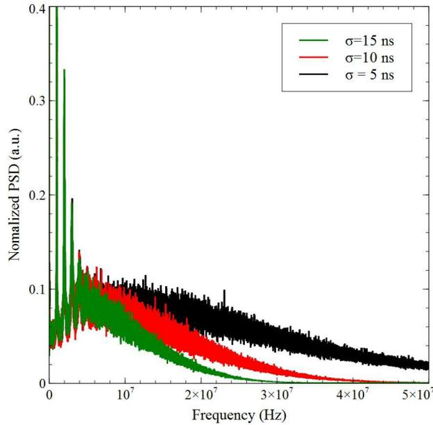
Figure 8: PSD obtained with simulated pulse trains.
