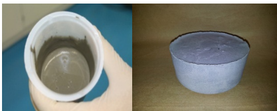
Fig. 3: Tritiated concrete before and after 3 weeks drying.
