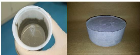
Fig. 3: Tritiated concrete before and after 3 weeks drying.
