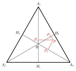
Fig. A.1. Lamé's coordinates of point P in the equilateral triangle are such that  $u = A_1P_1 - 2r$ ,  $v = A_2P_2 - 2r$ , and  $w = A_3P_3 - 2r$  (r being the inradius of the triangle and  $P_1$ ,  $P_2$ , and  $P_3$  being, respectively, the orthogonal projections of P onto  $A_1H_1$ ,  $A_2H_2$ , and  $A_3H_3$ ). Examples are O(0, 0, 0),  $A_1(-2r, 0, 0)$ , and  $H_1(r, -r/2, -r/2)$ .
