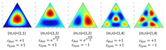
Fig. 3. Some eigenfunctions of the Laplacian operator in the equilateral triangle.
