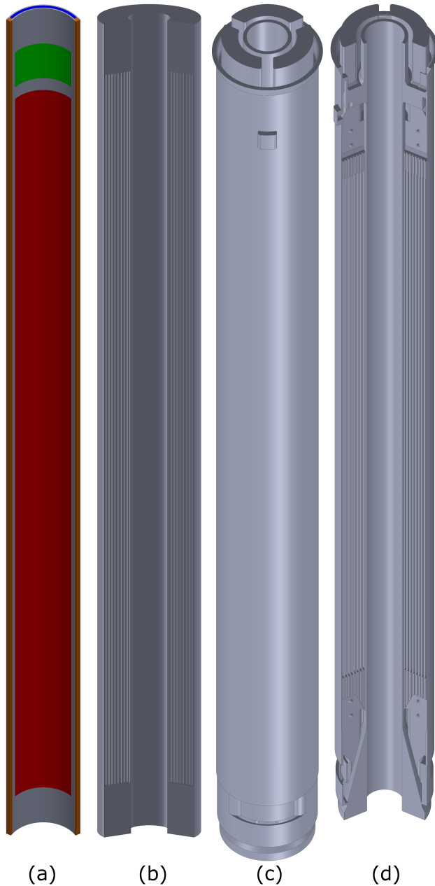
Figure 2: Isometric view of the following geometries: (a) the hot channel's assembly (water + metal), (b) the water between the fuel plates with simplified annular inlet and outlet (2/3 cut view), (c) the water between the fuel assembly and the rack and its 2/3 cut view (d). Sub-figures are out of scale.
