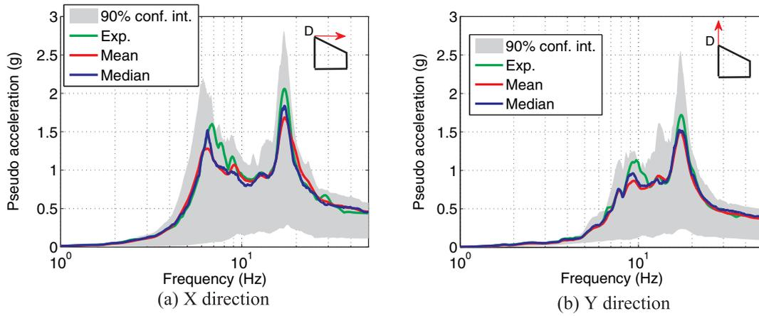
Fig. 8. Experimental/numerical comparison of the FRS – third floor – point D – run #7.
