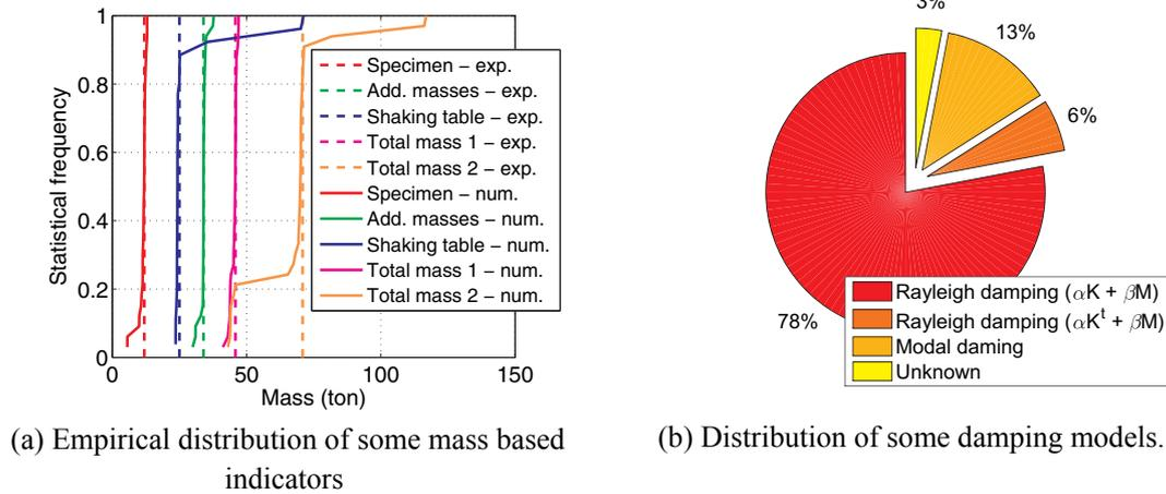
Fig. 4. Modeling assumptions – mass based indicators and damping models - Total mass 1 = overall mass of the RC specimen with the additional mass and without the mass of the shaking table; total mass 2 = overall mass of the RC specimen with the additional mass and with the mass of the shaking table.
