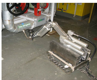
Figure 12: RICA robot equipped with a temperature detector during an intervention
