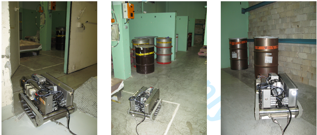
Figure 14: RICA entering (left) - advancing (center) - positioning in front of a drum (right)
