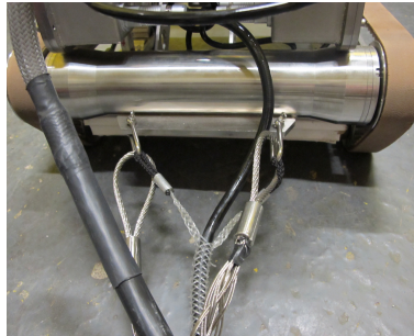
Figure 4: Stress take-up system attached to the RICA robot body
