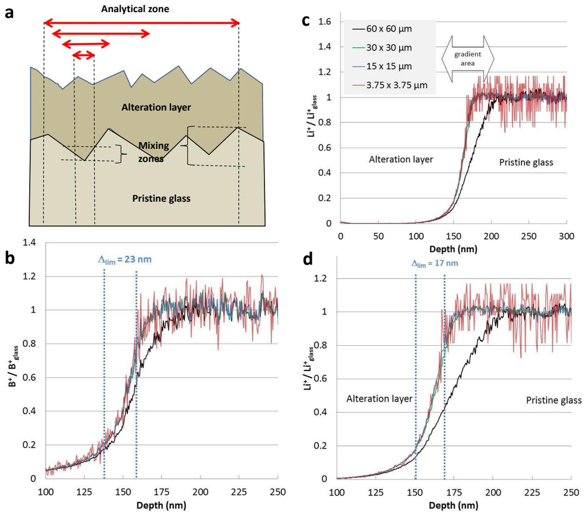
**Figure 2:** TOF-SIMS analysis of 180 day monolith. Chemical profiles are calculated in areas of  $30 \times 30 \mu\text{m}$ ,  $15 \times 15 \mu\text{m}$ ,  $7.5 \times 7.5 \mu\text{m}$  and  $3.75 \times 3.75 \mu\text{m}$  within the  $60 \times 60 \mu\text{m}$  area for boron (b) and lithium (c, d). This helps identify the existence of a mixing zone due to a rough interface or an uneven alteration layer (a).
