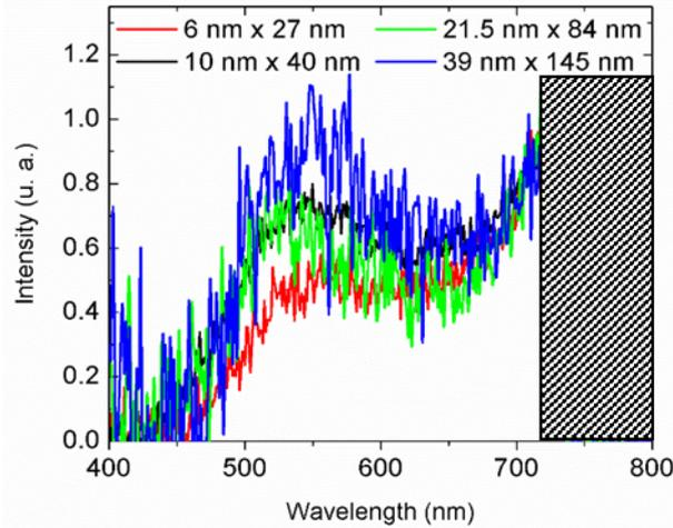
**Figure 2:** TPL spectrum of single GNRs: 6 nm x 27 nm (red), 10 nm x 40 nm (black), 21.5 nm x 84 nm (green) and 39 nm x 145 nm (blue). The hatched area corresponds to a non-measurable spectral range given the filters used to block laser excitation at the detector.
