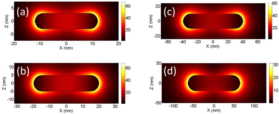
**Figure SP5:** Calculated electrostatic field enhancement map in intensity (*i.e.*  $f_{loc}^2-e_{xc}$ ) for each GNR simulated with BEM : (a) 6 nm x 24 nm (b) 10 nm x 40 nm (c) 20 nm x 80 nm (d) 40 nm x 130 nm. The excitation wavelength is equal to the longitudinal resonance wavelength of each GNR (793 nm, 799 nm, 828 nm and 820 nm respectively) and the incident polarization is along the long axis of the GNR.
