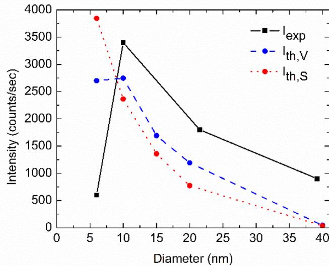
**Figure 5:** Experimental TPL intensity data (dark squares) and simulated TPL intensity resulting from the proposed model, considering either integration over the whole particle surface ( $I_{TPL,S}$ , red dots) or a bulk process ( $I_{TPL,V}$ , blue dots). An extra point corresponding to a GNR 15 nm x 60 nm was calculated (see figure SP9 for detailed BEM calculations).
