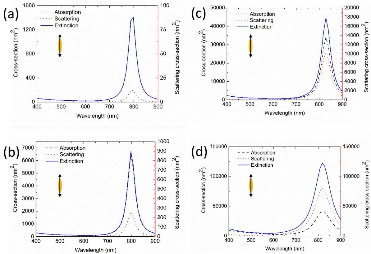
**Figure SP7:** Extinction (blue line), absorption (black dashed line) and scattering (red dotted line, corresponding to the right scale) cross-section calculated with BEM in retarded mode for each GNR (a) 6 nm x 24 nm (b) 10 nm x 40 nm (c) 20 nm x 80 nm (d) 40 nm x 130 nm for an incident polarization along the long axis of the GNR.
