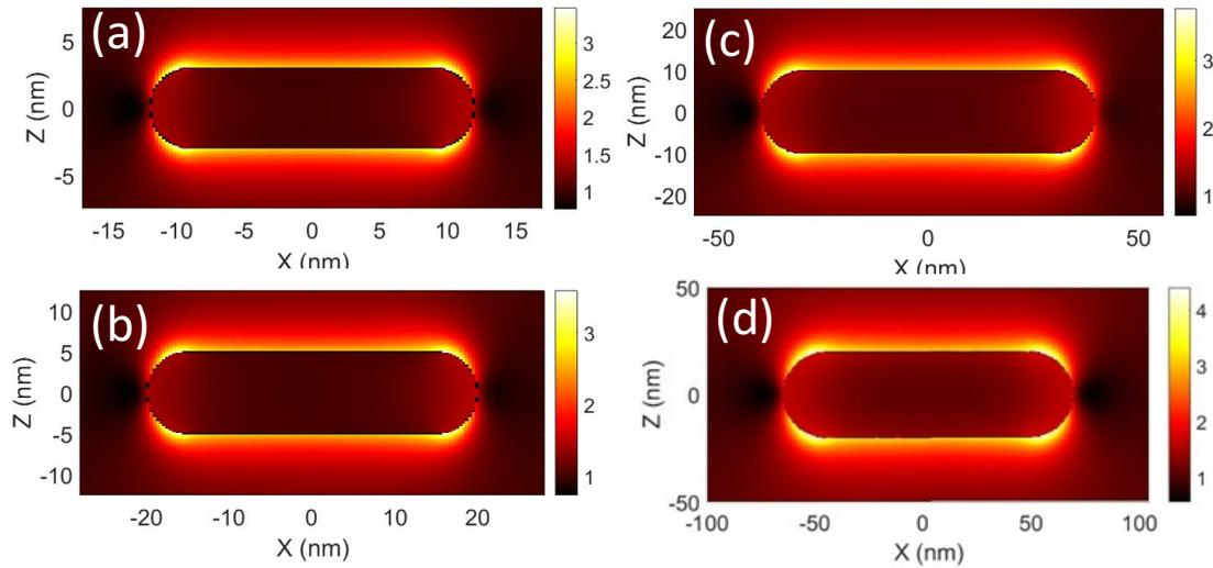
**Figure SP6:** Calculated electrostatic field enhancement map in intensity (*i.e.*  $f_{loc}^2-TPL$ ) for each GNR simulated with BEM (a) 6 nm x 24 nm (b) 10 nm x 40 nm (c) 20 nm x 80 nm (d) 40 nm x 130 nm. The excitation wavelength is equal to the transverse maximum scattering wavelength of each GNR (522 nm, 522 nm, 522 nm and 534 nm respectively – see figure SP8) and the incident polarization is along the short axis of the GNR.
