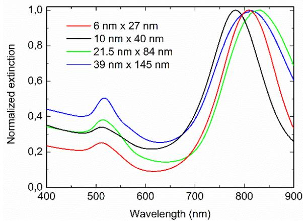
**Figure SP1:** Normalized extinction spectra of GNRs with respective diameters (d) and length (L): GNR1, d·L = 6 nm x 27 nm (red line, home-made particles see *Methods*); GNR2 : d·L = 10 nm x 40 nm (black line, home made particles, see *Methods*); GNR3, d·L = 21.5 nm x 84 nm (green line, *NANOPARTZ A12-25-808-CTAB*) and GNR4, d·L = 39 nm x 145 nm (blue line, *NANOPARTZ A12-40-808-CTAB*) in aqueous solution.
