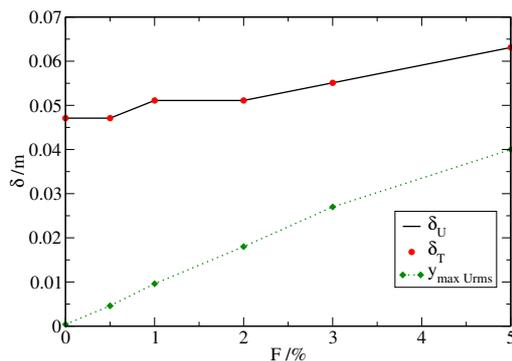
Fig. 10. Boundary layer thickness evolution with  $F$ .
