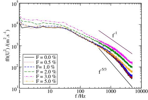
Fig. 23. Velocity spectrum at  $y = 31 \text{ mm}$ .
