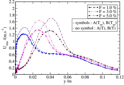
Fig. 6(a). Velocity fluctuations with instantaneous or mean temperature correction for  $A$  and  $B$ .
