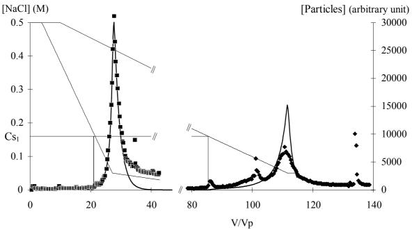
**Figure 3**: Comparison of particle release between simulation (——) and typical experiments with small and large V<sub>g</sub> values. The NaCl concentration (——) of the feed solution is decreased from  $C_i = 0.5$  M to  $C_f = 0.05$  M with  $V_g = 23.3$  V<sub>p</sub> ( $\blacksquare$ ) or with V<sub>g</sub> = 107 V<sub>p</sub> ( $\blacklozenge$ ).
