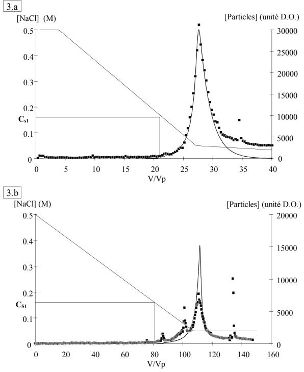
**Figure 3** *(details)*: Comparison of particle release between simulation (——) and typical experiments with small and large V<sub>g</sub> values. The NaCl concentration (——) of the feed solution is decreased from  $C_i = 0.5$  M to  $C_f = 0.05$  M with V<sub>g</sub> = 23.3 V<sub>p</sub> ( $\blacksquare$ ) or with V<sub>g</sub> = 107 V<sub>p</sub> ( $\blacklozenge$ ).
