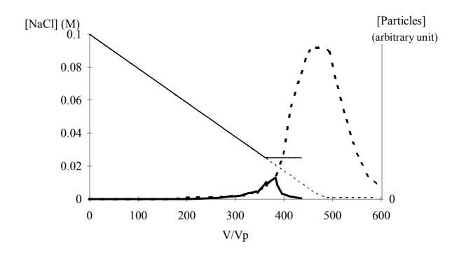
**Figure 1**: Effect of the final concentration,  $C_f$ , on the amount of particles leaving the column. The NaCl concentration of the feed solution is decreased to 0.001 M in column 1 (-----), while in column 2, the NaCl concentration is just decreased from 0.1 M to 0.025 M (---). As long as the NaCl concentration is the same, the particle breakthrough curves are identical (column 1 - - - -, column 2 -----).
