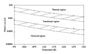
Fig. 1. Pyrolysis regimes versus temperature and particle size.
