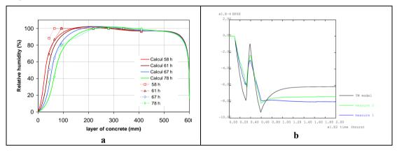
**Figure 4.** Comparison of predicted relative humidity in the layer of concrete versus measurement at different moments (a) and model predicted vertical strain versus measured strain on the heated surface (b)
