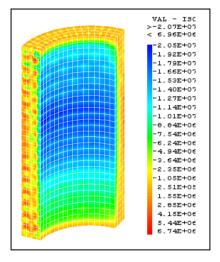
**Figure 8.** Reinforcement effect on  $\sigma_{zz}$  stress (in Pa)
