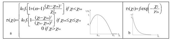
**Figure 3.** Hardening law in compression (a) and in tension (b)
