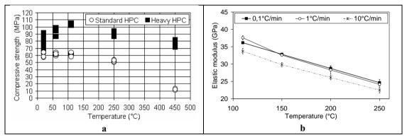
**Figure 2.** Evolution of compressive strength with temperature for standard and heavy HSC (a) and effect of heating rate on elastic modulus for standard HSC (b) <sup>[8, 9]</sup>
