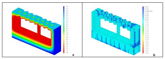
Figure 7. Vault's temperature field in normal way (a) and cracking due to tensile force (b)
