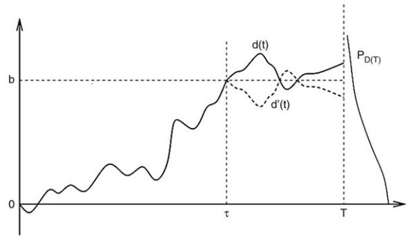
Fig. 3. Example of equiprobable time-histories leading to failure.
