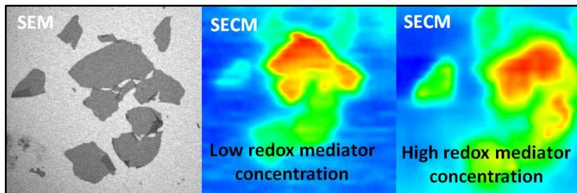
**Figure 1.** Presentation of the combined SEM-SECM responses at the basis of the advanced electronic conduction characterization.<sup>5</sup>
