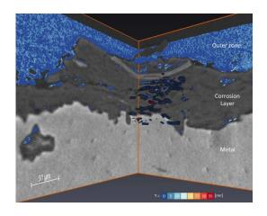
**Fig. 1** Water percolation of the porosity over time (blue: immediate, red: 30-35 minutes) in the corrosion layer of an iron rebar from the cathedral of Metz. Red zones show pores not directly connected to the main porosity network, where water percolates only in a second stage.
