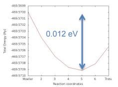
**Figure 1:** Equilibrium energy of CsPbl<sub>3</sub>'s orthorhombic phase (T<530K) for 7 sets of atomic positions obtained by DFT. The 5 intermediate position sets are linearly interpolated between sets 1 (*Moeller*) and 7 (*Trots*) which are equilibrium positions relaxed from experimental data<sup>3,4</sup>. The very flat profile indicates potentially low values for acoustic phonon modes.
