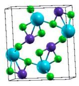
**Figure 2:** Equilibrium structure of CsPbI<sub>3</sub> in its orthorhombic phase for position set 5. The atomic positions are relaxed, and the blue, purple and green atoms respectively denote Cs, Pb and I.
