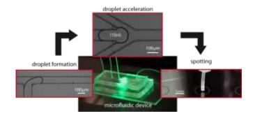
Figure 1. Principle of the droplet formation and MALDI deposition
