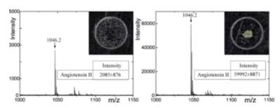
Figure 2. MALDI spectra. *Left*. Standard pipette deposit. *Right*. Microfluidic platform deposit. Inserts: Dried mixture of peptide/matrix before laser desorption.
