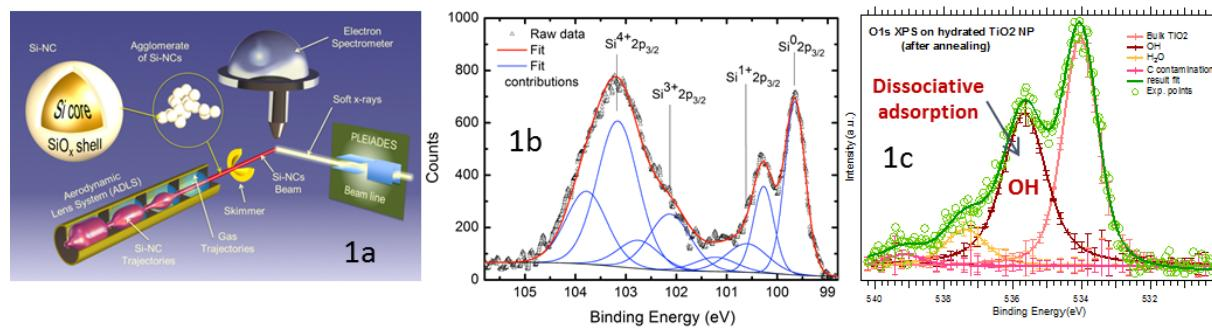
**Fig. 1a.** XPS of isolated nanoparticles. **Fig 1b.** Si2p XPS spectrum of isolated silicon nanocrystals. **Fig 1c.** O1s XPS spectrum of hydrated TiO<sub>2</sub> nanoparticles.
