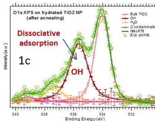
**Figure 1a.** XPS of isolated nanoparticles. **Figure 1b.** Si2p XPS spectrum of isolated silicon nanocrystals. **Figure 1c.** O1s XPS spectrum of hydrated TiO<sub>2</sub> nanoparticles.
