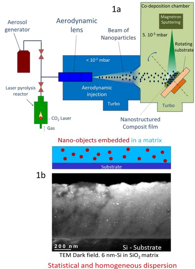
Figure 1a. General scheme of the co-deposition process.
