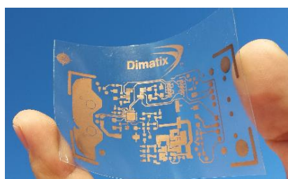
Figure 1: Copper patterns obtained on flexible substrate by electroless process after the primer printing, light-induced grafting and metallization steps.
