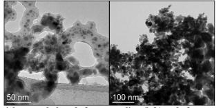
Figure 1. Particles morphology before annealing (left) and after annealing (right) Electrodes were then prepared using  $ZnFe_2O_4/C$  (70% wt.), CMC (12% wt.) and carbon additives (VGCF 9% wt., carbon black 9% wt.) to be cycled vs. lithium metal and postmortem SEM was done to observe the electrodes morphology after cycling.
