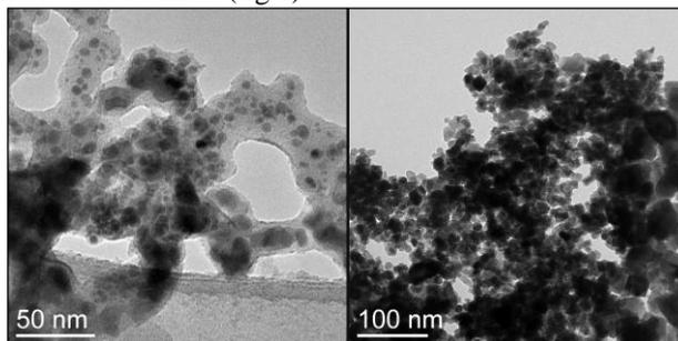
**Figure 1. Particles morphology before annealing (left) and after annealing (right)**
