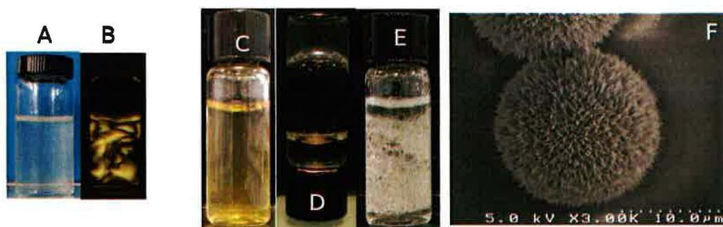
**Figure 1:** A) Water suspension of hybrid imogolite nanotubes with internal hydrophobic nanocavity, B) A observed between cross-polarizers, C) encapsulation of pyrene in water through hybrid imogolite, D) oil-triggered hydrogel formation, E) stabilization of an oil-in-water emulsion, F) electronic microscopy image of a dried water-in-oil emulsion droplet.
