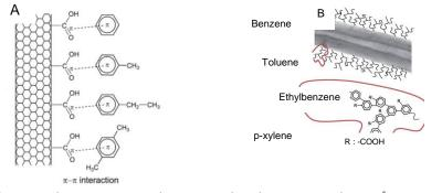
*Figure 1:* (A)  $\pi$ - $\pi$  stacking interactions between carboxylic groups and BTEX<sup>5</sup>, (B) Poly(phenylene) derivative grafted onto CNTs.
