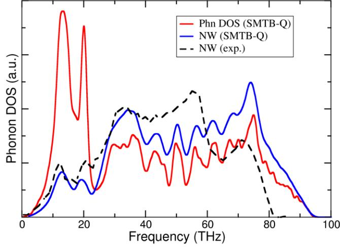
Figure 1 :Phonon density of states calculated with SMTB-Q (in red), neutron weighted phonon density of states calculated with SMTB-Q (in blue) compared to experiments extracted from Pang et al[44].
