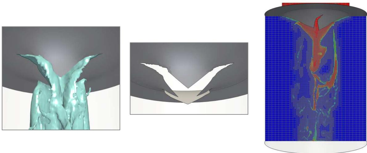
803 **Figure 28:** Water jet interacting with the cracks in the specimen and fluid mesh adaptation
