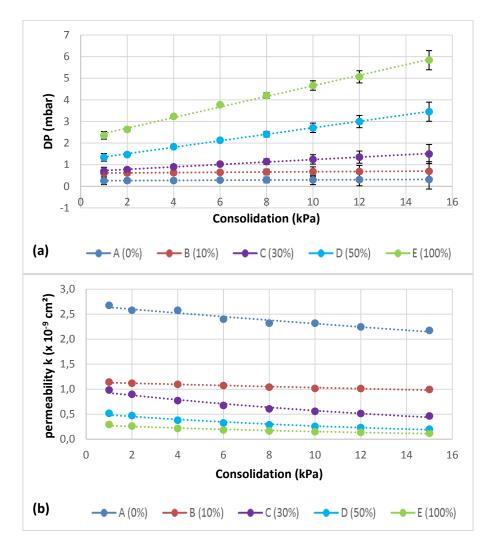
Figure 9 : Evolution of DP (a) and permeability k (b) as function of consolidation for different quantities of fines.
