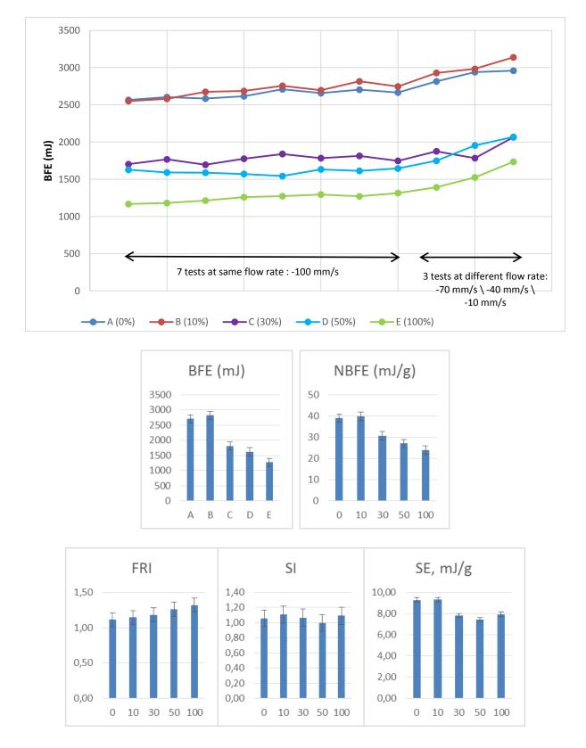
Figure 11 : VFR tests and the different indexes as function of quantity of fines (BFE, NBFE, FRI, SI and SE).
