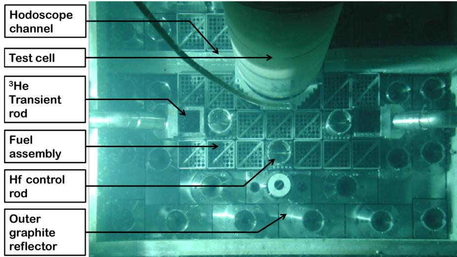
Figure 1: Radial cut of the CABRI reactor core
