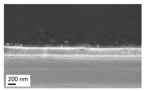
Figure 2: SEM micrograph of a nanocomposite coating of gold nanoparticles embedded in a silica matrix.
