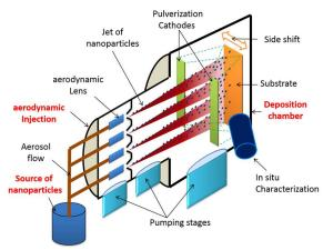
Figure 1: General scheme of the co-deposition prototype for large-surfaces.
